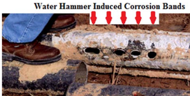
Figure 19. Evidence of Pressure Bands and Fatigue Induced Corrosion (Adapted from Leishear [3]).
