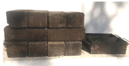
Figure 3. Manufactured Plastic Sand Bricks and mold.
