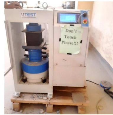
Figure 13. Compressive strength test by UTM.
